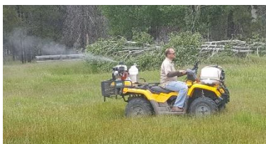
Photo 6 ATV Mounted Fogger
